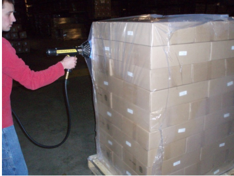
Step 2: If possible, tuck bottom of bag under or around the skid and then heat shrink.
